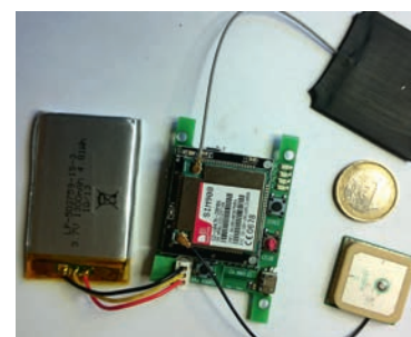
▲ Multichannel GPS tracking device for monitoring animal positions.
